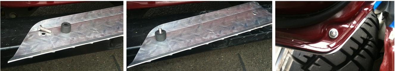
3. Next, install the lower door armor panel utilizing a 1" long screw, a flatwasher, and a nylock nut. Use the 1/2" long screws into the four square plastic inserts. Lightly tighten these screws to allow for a bit of alignment adjustability before final tightening.
