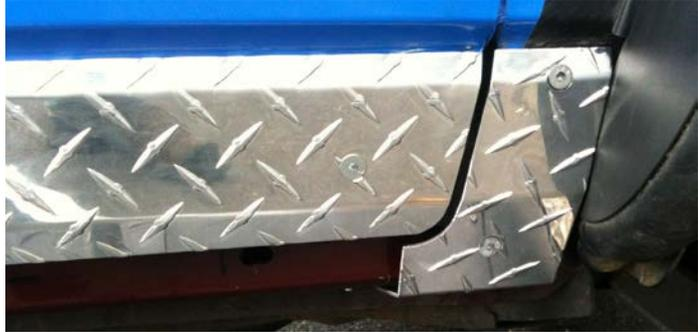
5. Proceed with installing the rocker armor. Line up the tabs in the rocker with the oblong holes in the FJ's body. Insert the tabs and push the rocker piece forward until tabs fully engage within the oblong holes.
