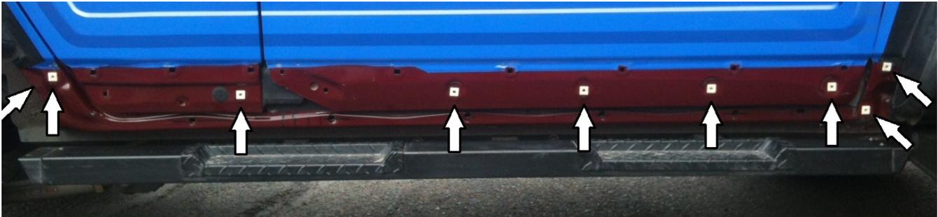
2. Begin the install with the rear access door panel. The rearward hole utilizes a 1" long screw, a rubber snubber, a flatwasher, and a nylock nut. Place the screw through the hole and capture the snubber on the inner side, then set the threads through the hole on the door. You'll need a slight amount of alignment adjustability before the final tightening, so only lightly tighten this nut at the moment. Now thread a 1/2" long screw into the forward hole and lightly tighten.
