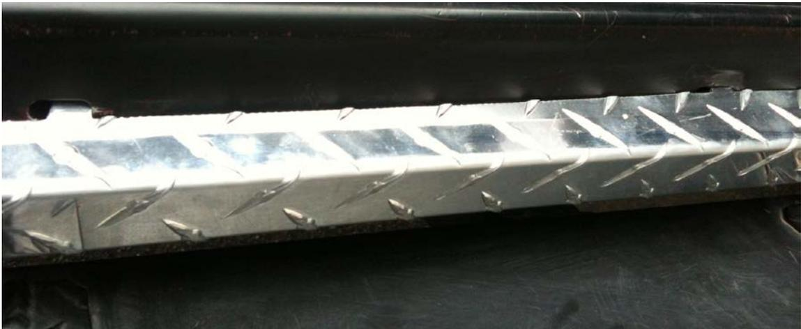
6. Once all the tabs are fully engaged, you should now be able to thread a ½" long screw into the square plastic insert at the rearward end of the rocker armor piece. Next, push in on the rearward end of the rocker armor piece towards the FJ's body until you can access the wheel well square plastic insert through the mounting tab on the rocker
