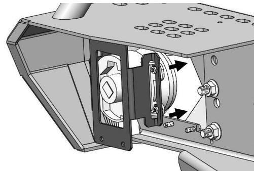
7. After the light passes through the opening, shift the mount bracket into place and slide it over the 4 threaded mounting posts.
