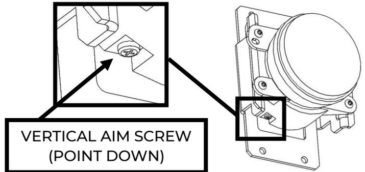
5. With the Phillips screw head pointing down toward the ground, insert the assembled fog light and mount bracket into bumper from the back side.
