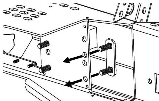
9. After all eight (8) Flange nuts are finger tight, verify the alignment of the bumper and completely tighten all of the Flange nuts.
