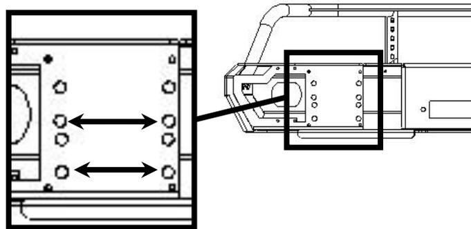
3. Prepare the Bolt Plates for installation by inserting two 1/2" Carriage Bolts through from one side.
