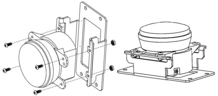
3. Before installing the light mount into the bumper, identify the top and bottom of the lights. When looking at the back of the fog light you will see a long Phillips head screw with a spring over it. (This screw is the vertical aim adjustment.)
