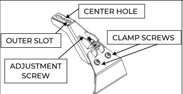
4. Prepare the mounts for installation by loosening the Clamp Screws (2 per mount) and the Adjustment Screw (1 per mount) so that the mount will open enough to fit over the rain gutter of the vehicle. Please note that in some cases the mounts may need to be partially disassembled in order to place the mount clamp over the rain gutter.
