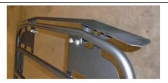
3. Position Air Dam so that there is a constant gap size between the Air Dam skin and the leading tube of the platform rack (figure 13). Fully tighten all hardware once you are happy with the position/gap. (This gap will provide clearance at the front tube for ropes, straps, and hooks to secure your load. The gap will be approximately 3/4" with the Air Dam positioned completely forward in the mounting slots.)
