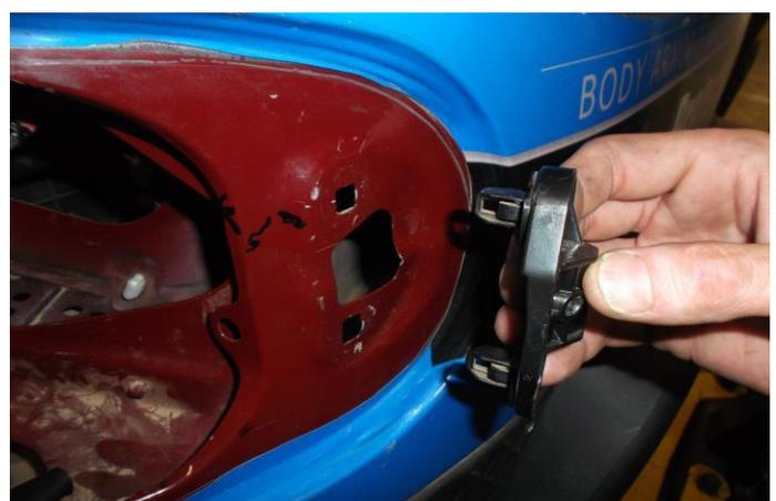
4. To prepare the wiring for the lights, the 5-wire to 4-wire converter must be installed. As mentioned above, it is your responsibility to choose which method you prefer for your wire connections and splices. To install the converter, you should remove the lower plastic threshold below the rear gate by removing the (5) Philips head screws, then gently pulling upward on the plastic trim starting at one end. This is where you can run wires across the vehicle. See Figure 7.
