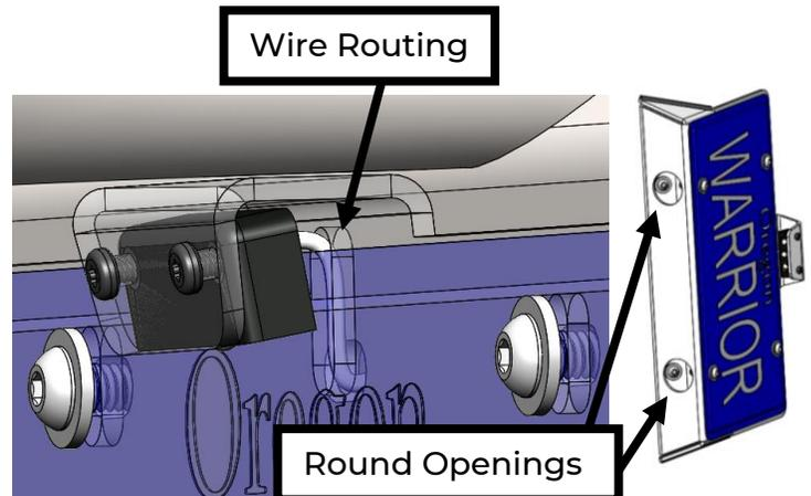
13. Visually align the license plate mount and tighten the bottom two screws first while holding the mount flat against the bumper face. After the bottom screws are tight, tighten the top two screws. (Remember to make sure the wires are not pinched between the license plate, mount, or bumper.)
