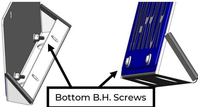
9. Before attaching the license plate and mount to the bumper, first install just the BOTTOM Button Head screws with washers and Nyloc nuts to attach the license plate to the mount (it is easier to attach before bumper installation).
