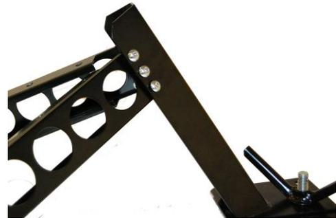
3. Locate the upper leg support plate (A). This will bolt onto the top of the support legs using four of the 1" Allen head bolts and lock nuts. Make sure when you install it that the bent tab at the top points up. Again, leave bolts loose until final assembly.
