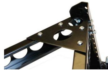
4. Install the tire support shaft (H) onto the assembly. This piece will slide down the inside of the main leg until the top hole in the threaded portion lines up with the top hole in the main leg. Use your 2" long allen bolt to bolt thru the main leg, the tire support shaft, and the vertical tab in the support leg top plate. Use your remaining 1" long Allen bolt through the bottom hole in the main leg where the tire support shaft aligns with it.
