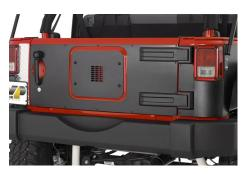
**IMPORTANT:** Warrior recommends the installation method of drilling holes and pop-riveting the tailgate cover into place. Any other method of attachment, gaskets or sealants used is up to the discretion of the installer. All covers are designed to overlay the existing factory tailgate with provisions for the factory hinges and latches.
