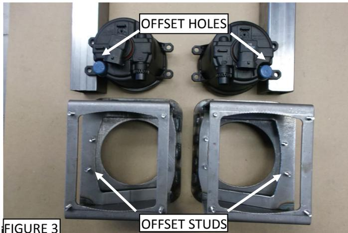
2. Carefully place a fog light into its corresponding light bucket. Make sure the fog light is seated properly and are not to scratch the clear lens of the light (follow the steps below and see **FIGURE 4**).
