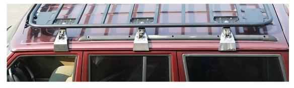
6. Loosely attach the basket/platform to the gutter mounts. Do not tighten hardware at this time. Check the position of the platform/basket to make sure the location is correct.
