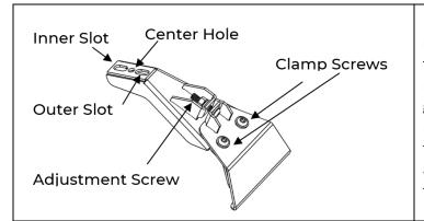
1. Prepare the mounts for installation by loosening the Clamp Screws (2 per mount) and the Adjustment Screw (1 per mount) so that the mount will open enough to fit over the rain gutter of the vehicle. In some cases the mounts may need to be partially disassembled in order to fit the mount clamp over the rain gutter. (If all mounts are not assembled, assemble them to match the figure to the left)
