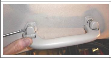
29. Now move to the front seats and remove the front grab handles. The removal process is identical to the rear grab handles (steps 14 – 16), but the front handles do not have an integrated luggage hook. Make note of this difference so that you know to put the handles with the luggage hook in the rear and the handles without the luggage hook in the front upon re-installation.
