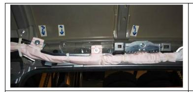
2. Move to the back seat and remove nuts #3, #4, and #5 as indicated. You should be able to leave the airbag in place while removing these nuts.
