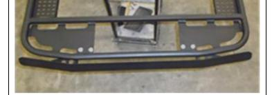
QUALITY INTEGRITY INNOVATION SERVICE 27. Gently place the platform on top of the mounts. Locate the platform by aligning the holes in the mounts with the appropriate slots in the platform bucket. Refer to the images and notes while inserting the bolts. Loosely insert all twelve 3/8" bolts and washers before tightening any hardware.
